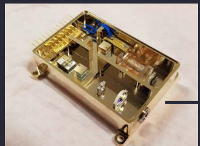
Frequency stabilised laser – 780nm (same wavelength as CD burner)
